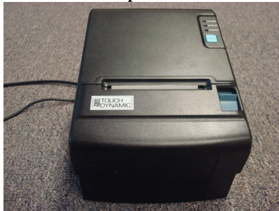
Ports: RJ11 (for Cash Drawer) Comm. Cable to Breeze: COM1 (for both WS01 and WS02)
